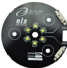
BAS13198: MCPCB+Cree LED (XPG)+Wango Connector
