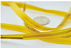
BFS11002: 1L FPC, size: 1510*7.5mm, ENIG, soldermask, T=0.05mm.
