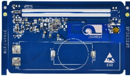
BPD13205: 0.15mm extra thin PCB + Components + Battery
