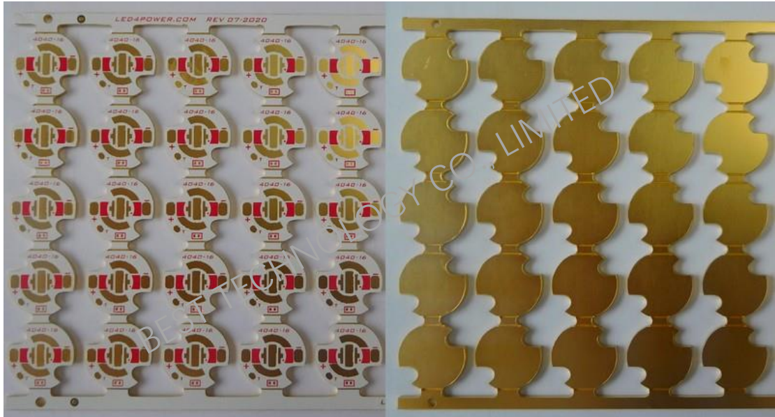
Top and bottom view of finished SinkPAD board- in panel)
